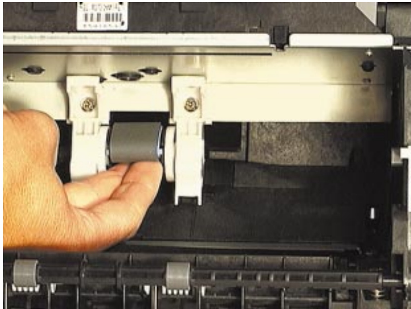
Figure 4-38 Changing the pickup roller
