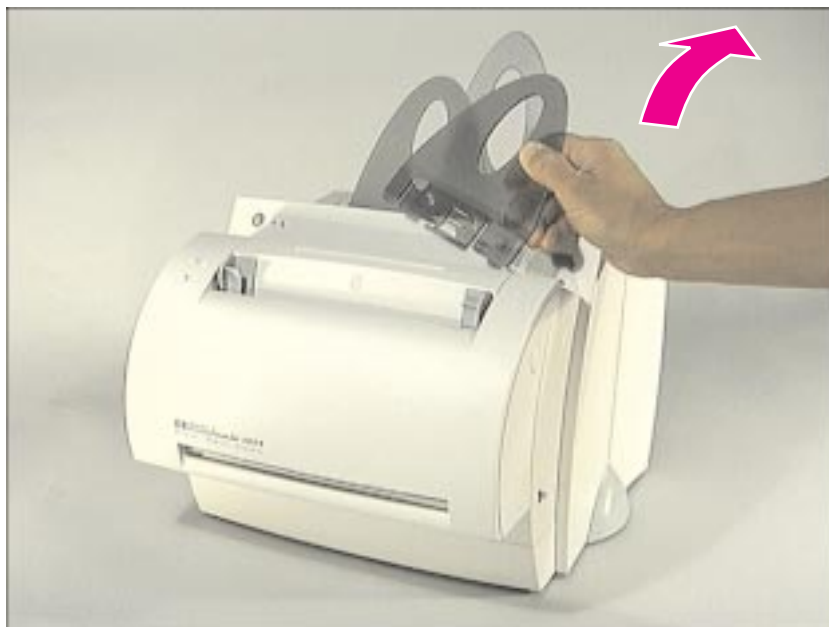
Figure 4-1 Removing the paper guides
