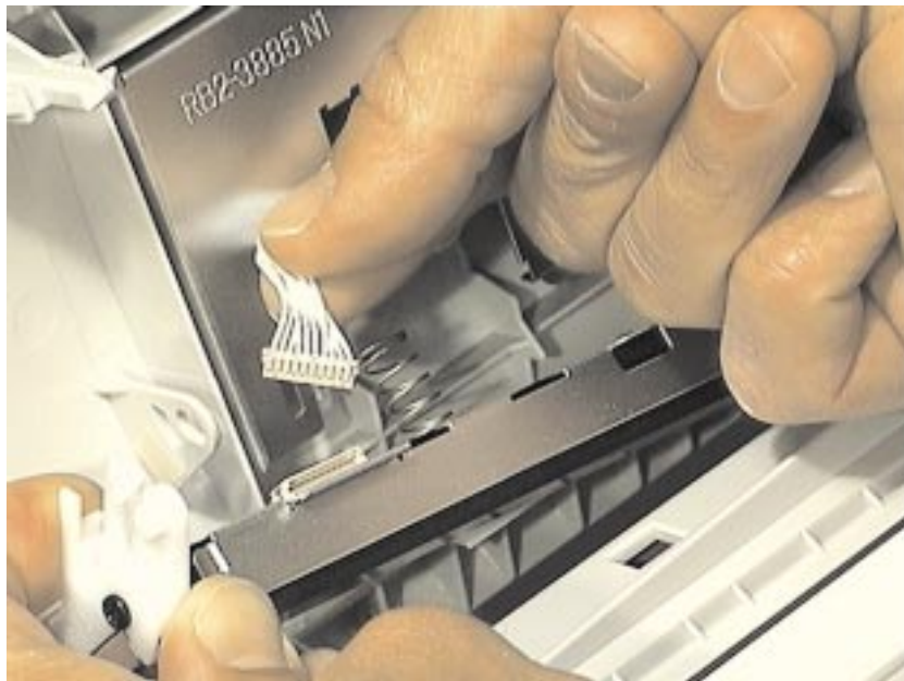
Figure 4-6 Disconnecting the CIS wire connector
